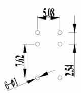
Remarks: (1) In case of no tolerance shown in outline dimension: outline dimension  $\leq$  1mm, tolerance should be  $\pm$  0.2mm; outline dimension > 1mm and  $\leq$  5mm, tolerance should be  $\pm$  0.3mm; outline dimension > 5mm, tolerance should be  $\pm$  0.4mm.
